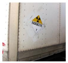
Placard Placement!?! Did you have to tilt your head a little to see this placard? Make sure your placards are in fact displayed horizontally per 49 CFR 172.516(c)(5). Also, does a placard need to contrast with its background? Hopefully, you said, "Yes!" If the placard does not contrast with the background, then we need to add an outer border per 49 CFR 172.516(c)
