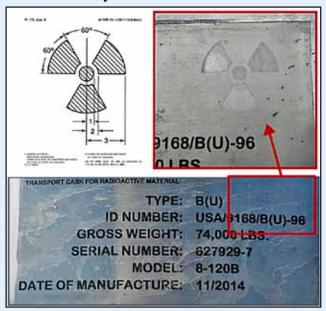
Should your Type B(U) packaging have a radiation symbol? Must this trefoil symbol be permanently engraved, embossed or stamped on an outermost receptacle and resistant to the effects of fire and water? Is there any specification to the symbol's size, shape and design? I hope you answered 'yes' to all these questions. This package marking is required in 49 CFR 172.310(d) and must be designed to the specifications in 49 CFR Part 172 Appendix B.
