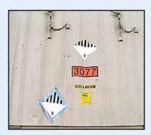
Placarding is a shared responsibility between both the shipper and the carrier per 49 CFR Part 172 Subpart F. Should the shipper place the placard where the driver can replace or cover
