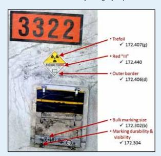
Lots of marking and labeling issues outlined in this picture. The trefoil and label must be designed to the specifications and requirements outlined in 49 CFR Part 172 Subpart E and Part 172 Appendix B. When a label is placed on a non-contrasting background, an outer dashed or solid line border must be added to the label. In addition to the orange panel, any other bulk markings must be of appropriate size and legible per 49 CFR Part 172 Subpart D.
